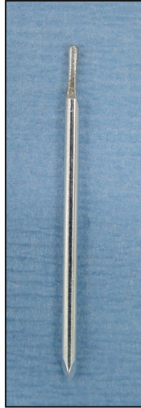
Figure 6.1: Image of the 316LSS pin implant used. Note how one end of the pin is hand milled so it had a smaller diameter.
