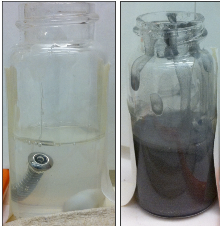
Figure 5.1: 316LSS screws being coated with PCL composite. The image on the left is PCL alone and the right is PCL+Mg-mesh.
