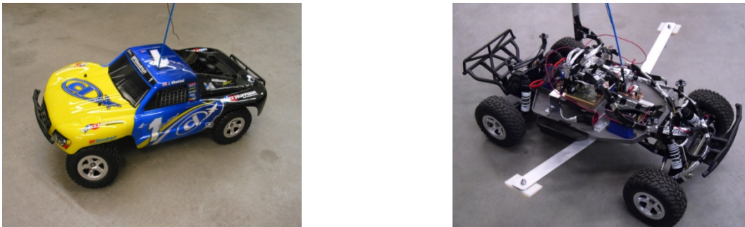
Figure 5.12: Scaled Test Vehicle: 1:8 (30.5 x 58.5 cm)
