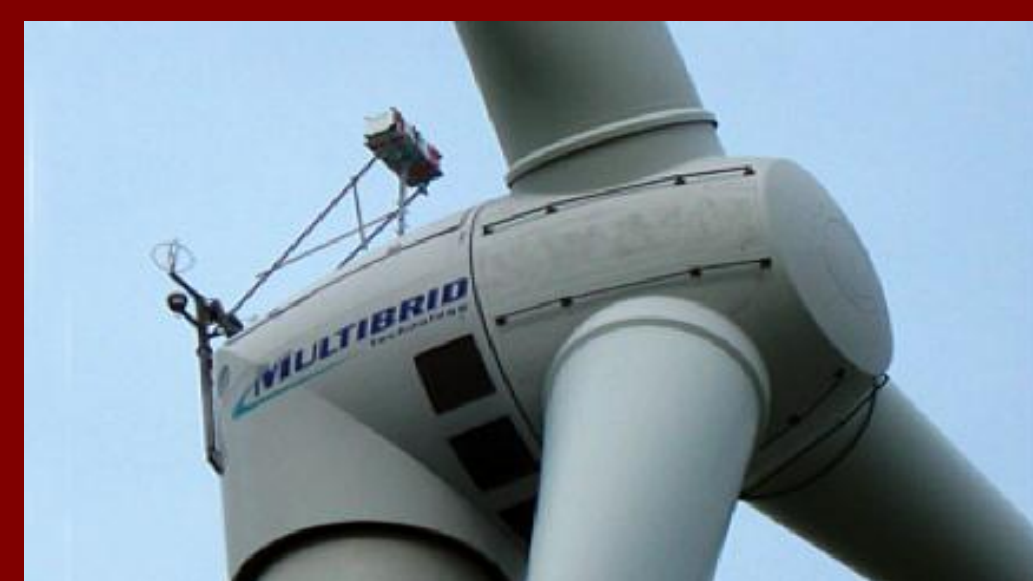
Figure 2: This image gives a visual of a LIDAR device mounted on a wind turbine [3].
