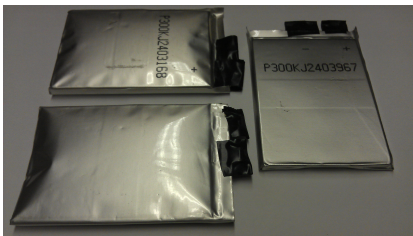
Figure 2.1: Left : Front and back sides of two bad (swollen) LiPB cells. Right : A normal cell of the same type.
