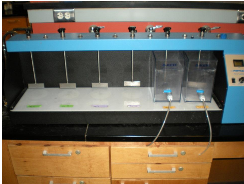
Figure L2: Phipps and Bird jar test apparatus used for all jar test experiments
