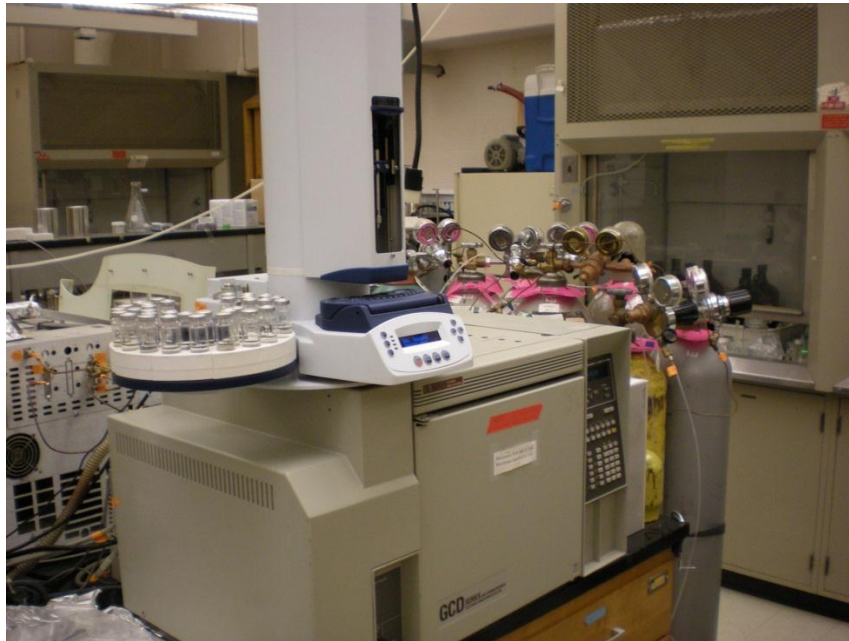
Figure L1: Image of HTA autosampler (top) and HP GC-MS (bottom)
