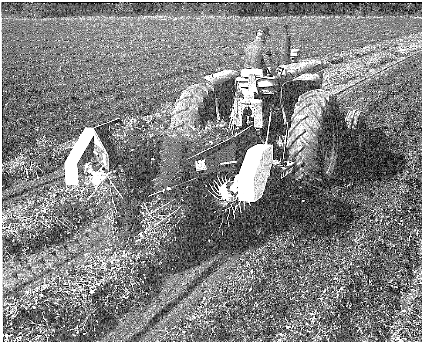
Figure 13. The inverting windrower catches the plants as they leave the shaker. Additional soil is sifted from the plants before the inverting rods form a windrow of plants with pods on top. (Courtesy Lilliston Corporation).
