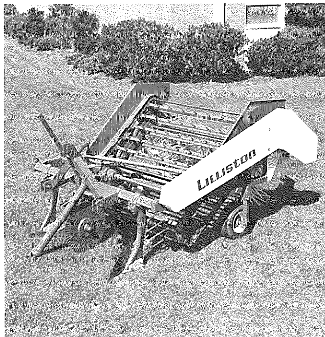
Figure 12. A two-row peanut digger-shaker-inverter showing blades that resemble plowshares and the shaking elevator which removes soil from the plants. (Courtesy Lilliston Corporation).
