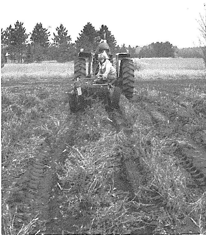
Figure 14. This potato digger used to harvest peanut plots simulates the digger-shaker portion of commercial peanut harvesting. The potato digger did an effective job when operated at one-half the depth used for potato. The addition of a windrow inverter at the rear would make the operation similar to that of modern commercial peanut production.
