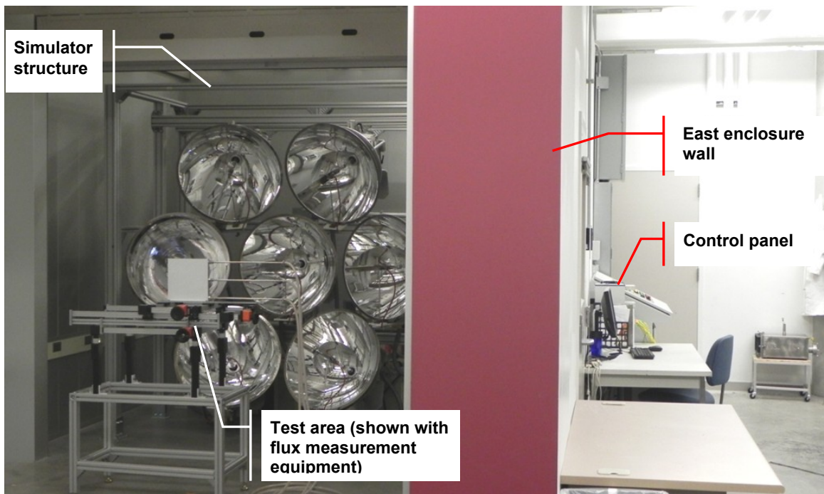
Fig. 4.1: Photograph depicting the final solar simulator fabrication, including the simulator support structure, enclosure, and control panel
