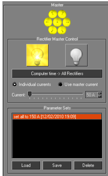
Fig. C.6: Screen shot of KEX Control 7 showing the master control of all seven units
