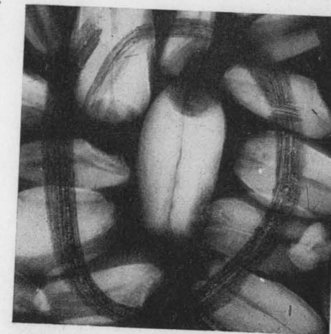
Fig. 3. The typical radiographic appearance of Laemophloeus sp. attack.
