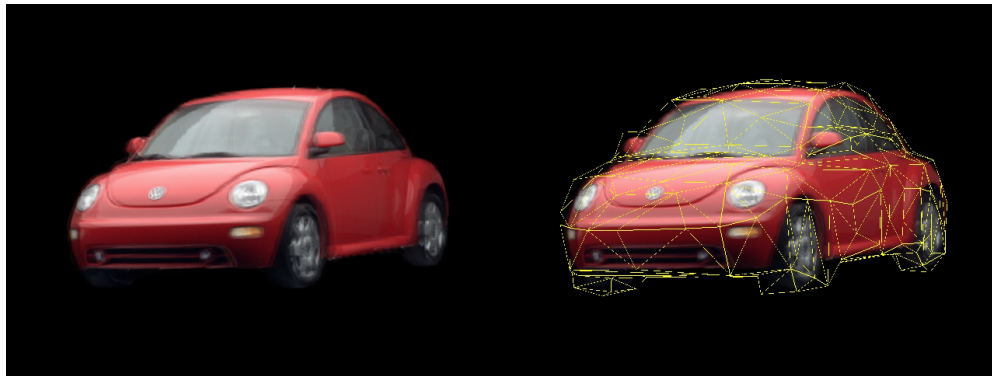
Figure 3.12: An unstructured lumigraph of a Volkswagen Beetle (left), and the proxy geometry used to render it (right). From [Buehler et al., 2001].
