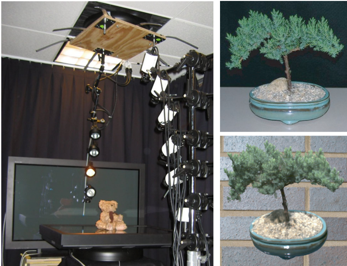
Figure 3.16: Setup and example rendering of work by Matusik et al. On left, the capture device used. On right, the top image is one of the original photographs while the lower image is rendered from the resulting light field. From [Matusik et al., 2002].
