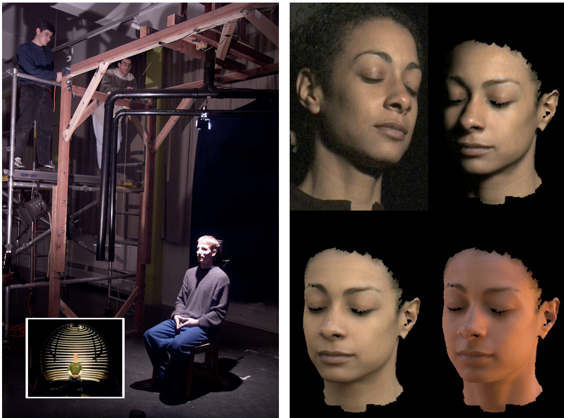
Figure 3.15: Setup and example rendering of work by Debevec et al. On left, the device known as Light Stage 1. On right, the top left image is one of the original photographs. The other three images are rendered from a unique angle using environment map lighting to relight the face. From [Debevec et al., 2000].
