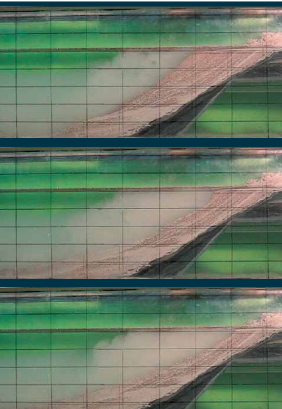
LEFT Laboratory experiments demonstrating delta-front landslide events. TOP: Before landslide MIDDLE: During landslide BOTTOM: After landslide
