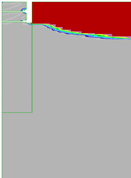
Figure 4.19: Contour of tensile strength for 5.6 \sigma_t (14 MPa).
