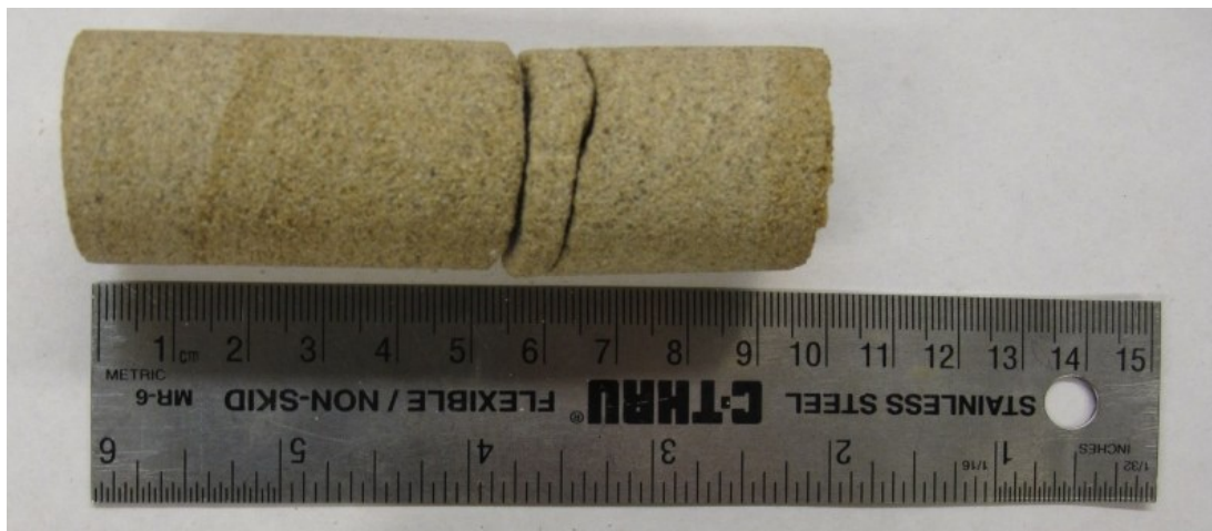
Figure 2.2: Photo of core diskings in Boise sandstone
