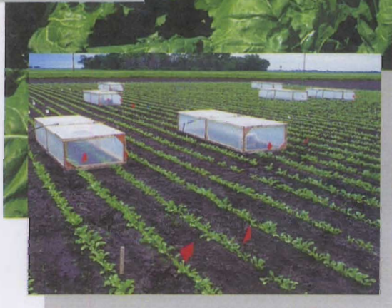
Weather enclosures enable investigators to study the effects of moisture, temperature and wind on weed control.
