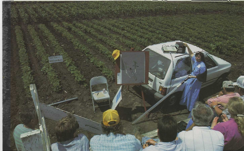
At an experiment station field day, Sister Esther Nickel explains to farmers how she videotapes in the ground. Long clear plastic tubes like the one she is holding are inserted in the soil next to corn and soybean plants very soon after planting. A video sensor is attached to a long pole with a light at the bottom, and lowered down each tube every week during the growing season to record root growth in place. Her presentations include an explanation of how her research on rotation effect may someday affect a farmer's production.
