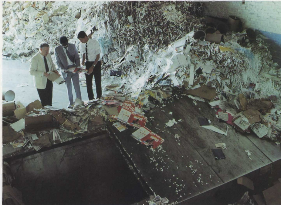
Forest Products department head Jim Bowyer, researcher Mutombo Muvundamina and Waldorf Corporation Technical Services Manager Gary Kaziukewicz (right to left) are with collected paper ready for a hydropulper. The paper is turned back into pulp using hot water and mechanical energy, and extensively screened and cleaned on its way to being remade into paper products. The St. Paul Waldorf plant, operating since 1906, makes paperboard from recycled fiber. Experiment station research seeks to help the paper industry overcome technical problems in the recycling process.
