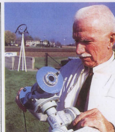
Donald Baker checks a pyrheliometer, which measures direct beam solar radiation, at the weather station.
