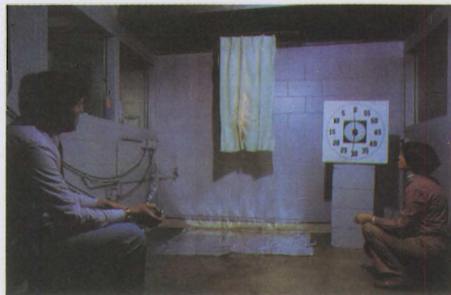
At 30 seconds after ignition the flames are climbing up the back of the drapery.
