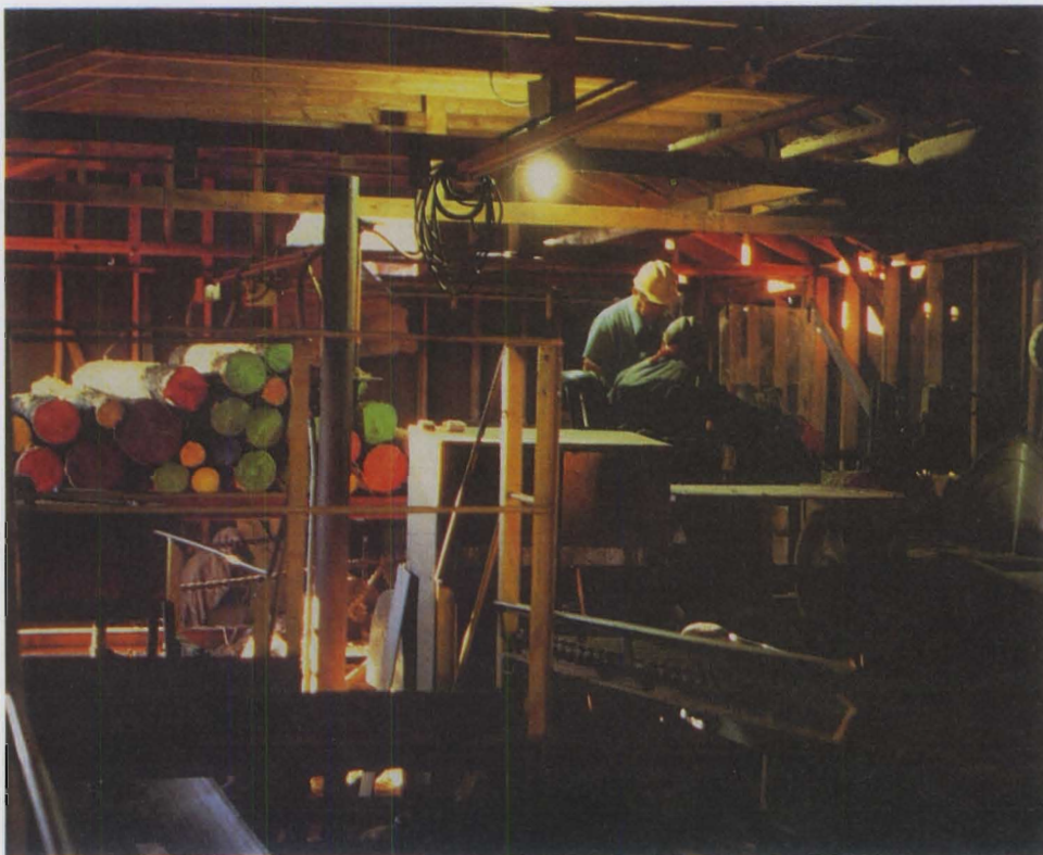
Above: Forest products scientist James L. Bowyer color codes the ends of logs from budworm-killed balsam firs of various diameters. Below: The color-coded logs were then milled into 2×4s and 2×6s at Latvala Brothers Forest Products, Nashwauk, Minnesota, enabling the University of Minnesota research team to determine the yield of dimension lumber from each tree size.
