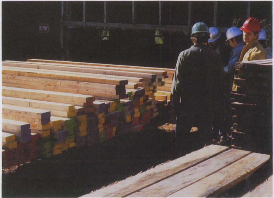
At Latvala Brothers Forest Products, Sinclair, Bowyer, and others inspect the lumber cut from the color-coded logs. The lumber was later graded by a chief inspector of the Northern Hardwood and Pine Manufacturers Association before being shipped to Kaufert Laboratory for strength tests.
