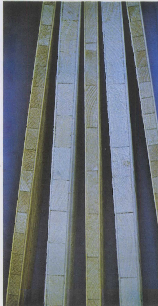
A cross section view of blockboard shows the use of native hardwoods laid edge to edge and overlaid with veneer (photo by Steven Sinclair).
