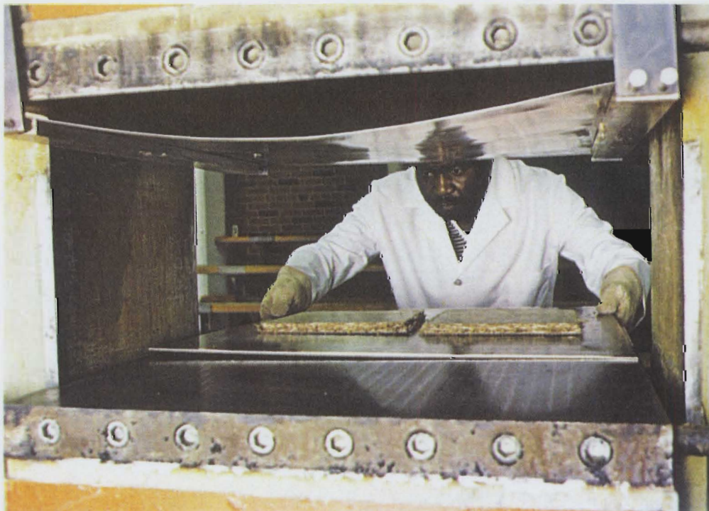
Samuel Okoro, research assistant, operates a hot press which is used for making particleboard in laboratory experiments (photo by Dave Hansen).
