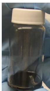
Figure 1.2 CZTS nanocrystals dispersed in toluene.
