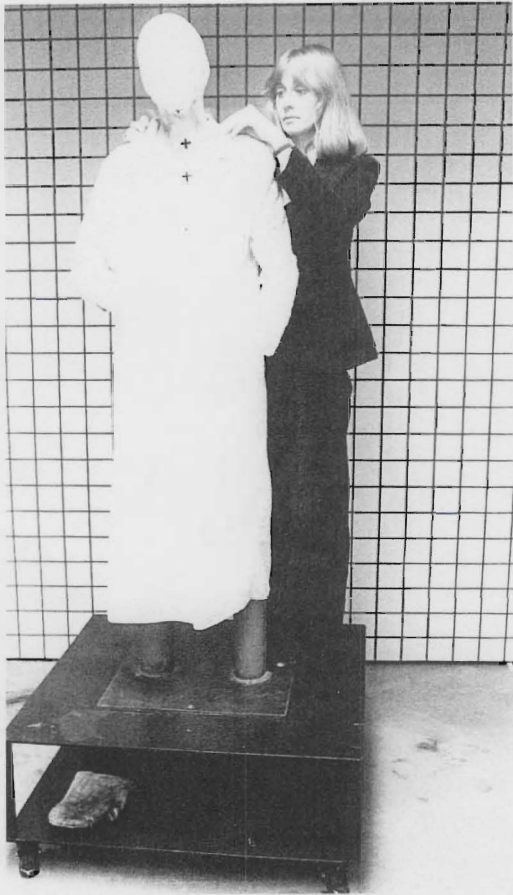
Graduate student Marjorie Norton adjusts garment before burning it on the instrumented mannequin. Crosses on mannequin indicate location of thermocouples.
