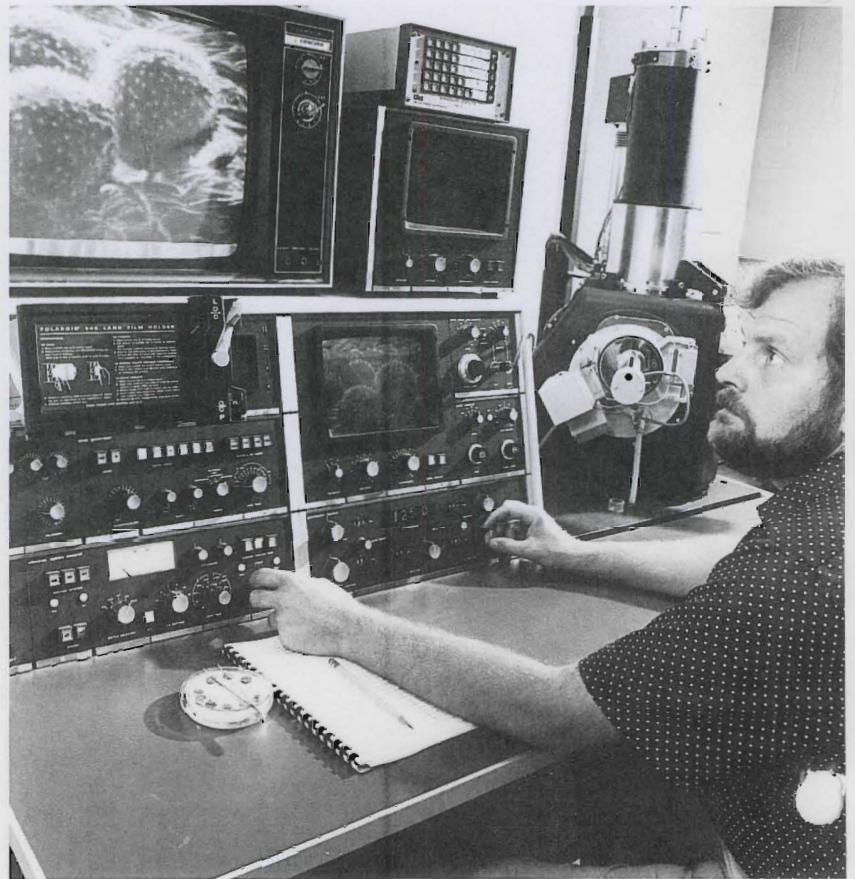
The scanning electron microscope projects the image of specimens being examined on a television screen while a camera can photograph the specimens, for example this dandelion pollen (above) and spider (above, next page).
