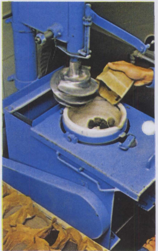
Above left: Small scoops are used to measure a specific volume of soil for the phosphorus and potassium analysis. above: Samples are ground fine enough to pass through a 10-mesh sieve. left: Electrodes are placed into a soil-water suspension to determine nitrate content.
