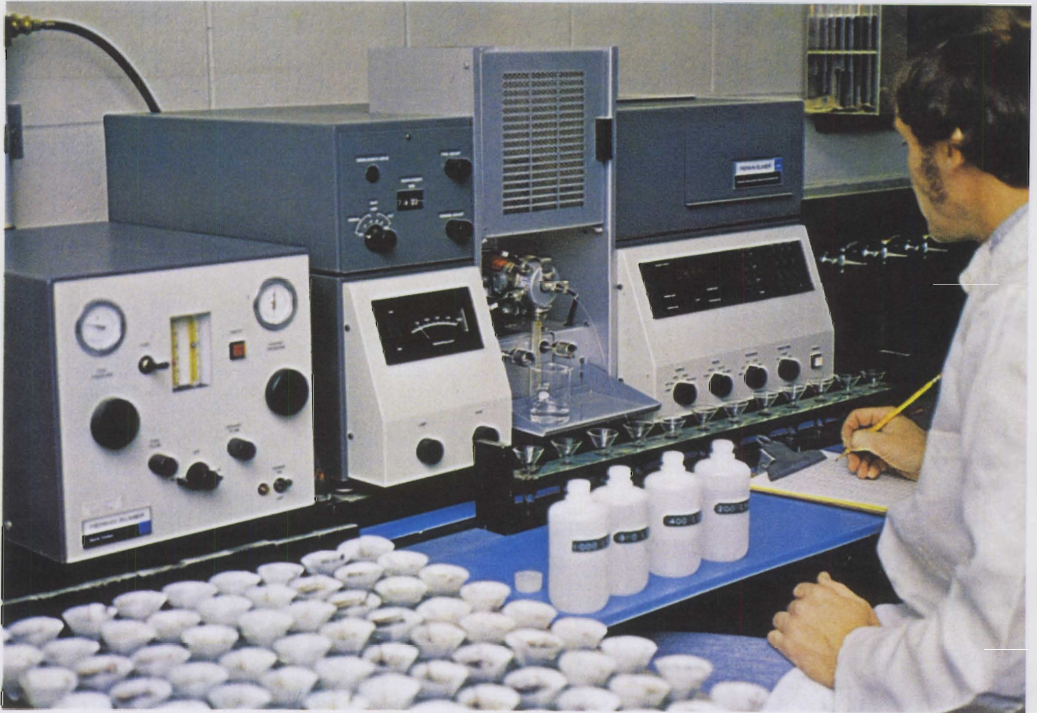
An atomic absorption spectrometer helps determine the potassium and zinc content.
