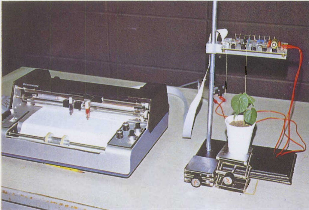
Continuous recording of leaf movements is accomplished with this electronic device (photo by Audrey Engels).
