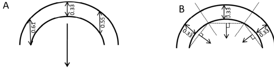
Figure 2.3: A) If only one vector is used to compare a curved bluff the change on the edges will be overestimated. B) When the bluff is broken into nearly planar areas, comparisons can be made more accurately. Three best fit planes are created for the curved sections of the bluff and vectors used for comparison are normal to these planes.
