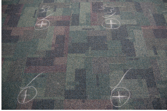
Figure 4.4: A portion of the floor that shows the manually placed marker positions roughly 1m. apart.
