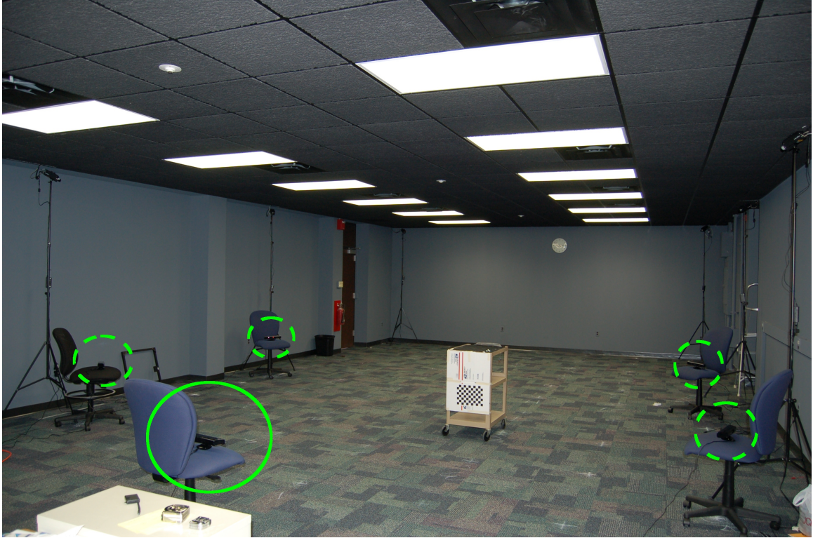
Figure 4.3: Figure shows multiple Kinects arranged in a typical VR Lab setup for a 360° coverage of a circular space of radius 3.5m. The solid green circle shows the active primary Kinect, while the dashed green circles show the passive secondary Kinets.
