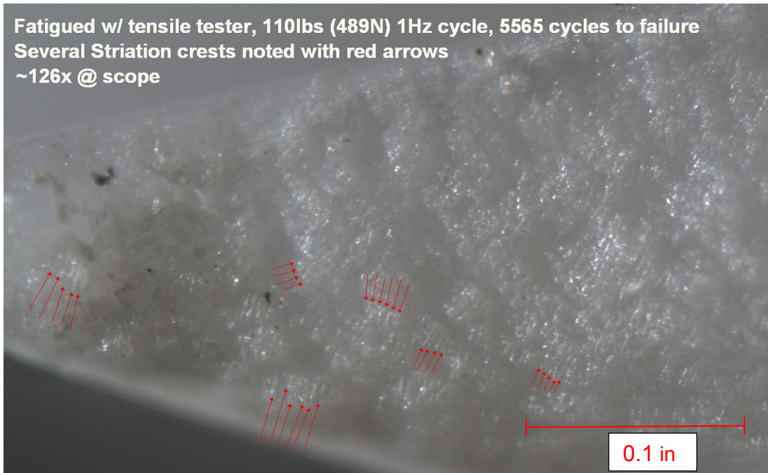
Figure 30: Optical micrograph of intentionally fatigued exemplar part.
