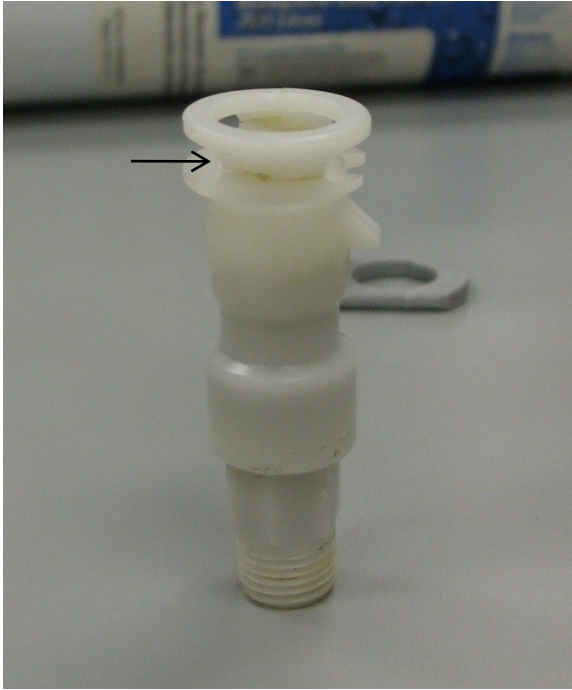
Figure 3: Photograph showing the location of the crack in the mode of interest to this analysis. The crack passes through the "ears" responsible for retaining the latching mechanism. An arrow indicates the crack location in the figure.
