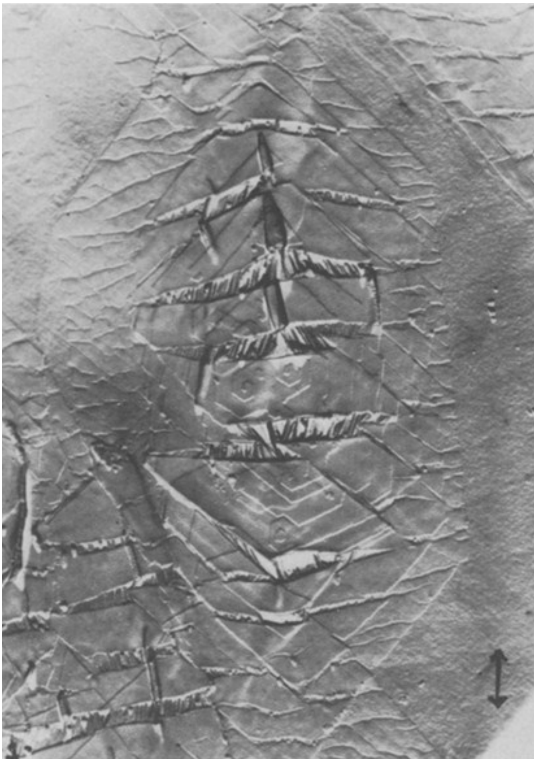
Figure 15: A crystal multilayered from spiral growth was fractured through deformation of 100% in the direction indicated by the arrow. (Gohil, Patel, & Patel, 1974)
