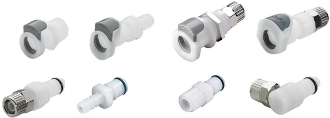
Figure 1: Exemplar APC couplings. A coupling consists of a male and female component, which are joined by a locking mechanism. Body (female) components are shown on the top row. Insert (male) components are shown on the bottom row.
