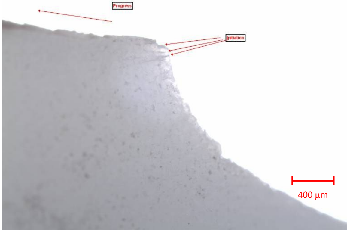
Figure 6: Optical micrograph of the initiation location at the end of the ear. Multiple cracks initiated at this location, one of which progressed across the entire fracture surface. These cracks would not have formed had the crack initiated in the center of the ear near the void, as the overall area when the crack reached this point would have been so small and the effect of the sharpness of the crack tip so large that the material in the plastic zone would simply have fractured, not generated additional, parallel cracks off-plane.
