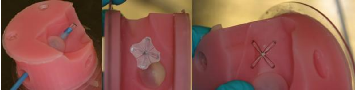
Figure 77 – 2 nd generation mold with SJM Premere device deployed
