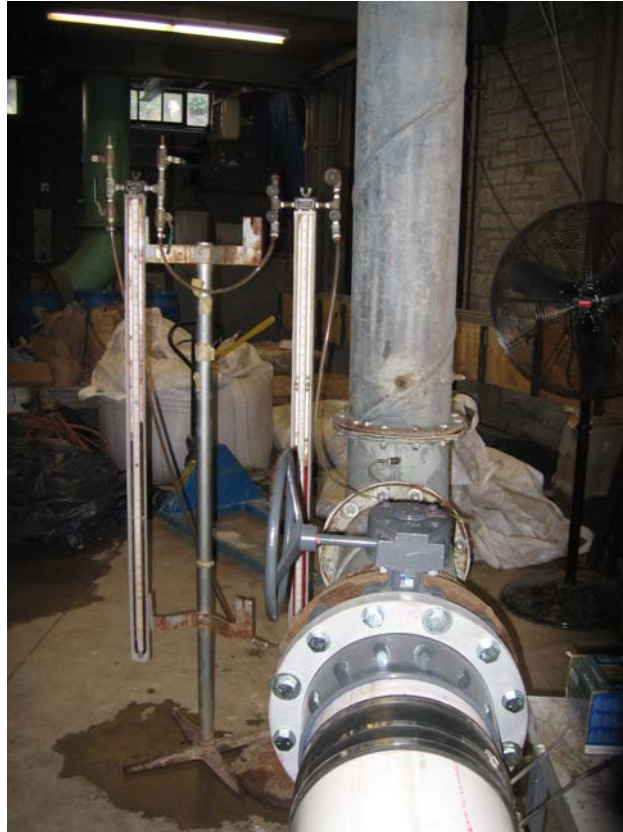
Figure 2.3. A Meriam manometer connected to pressure taps mounted on an elbow via plastic tubes.
