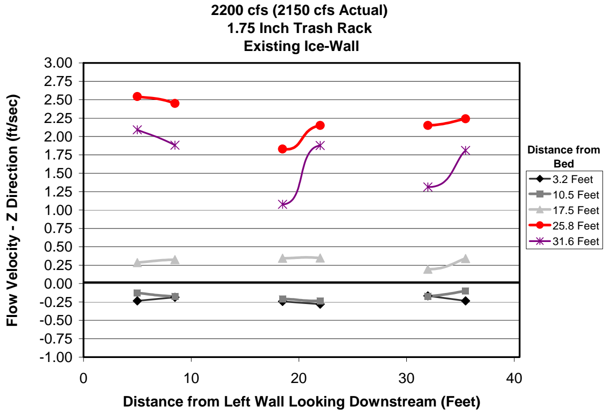
Figure C.7. The z-component of the velocity measured at 30 locations inside the bay areas, 2.9 ft away from a trash rack with 1.75-inch openings at its current location, under the 2200 cfs flow condition. The actual measured flow was 2150 cfs.
