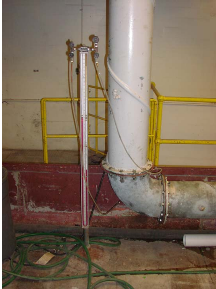
Figure 13. The elbow meter consisting of a Meriam manometer and two pressure taps on the 12-inch water supply line was used to measure the total flow rate.
