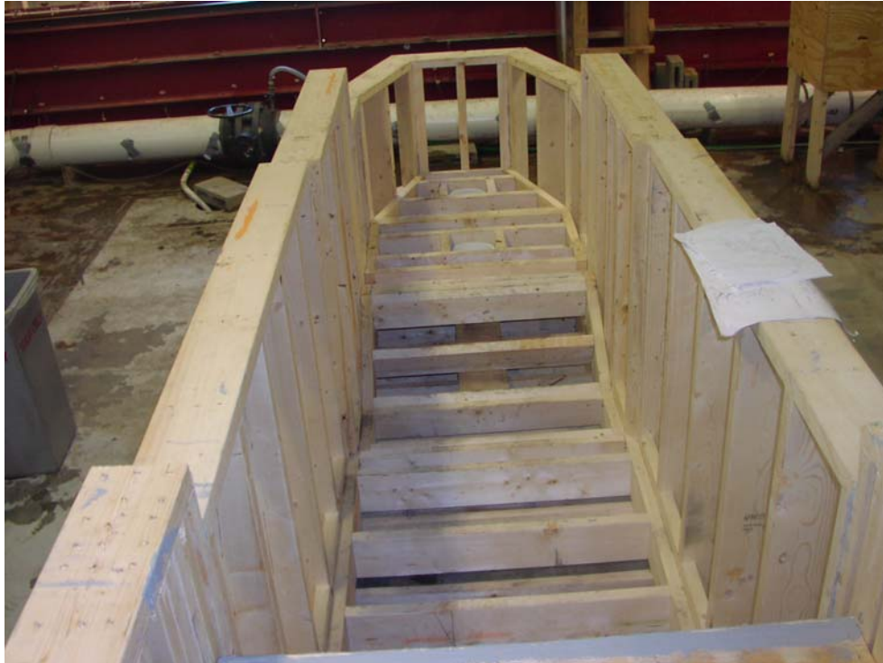
Figure 8. The model was built of plywood and lumber.
