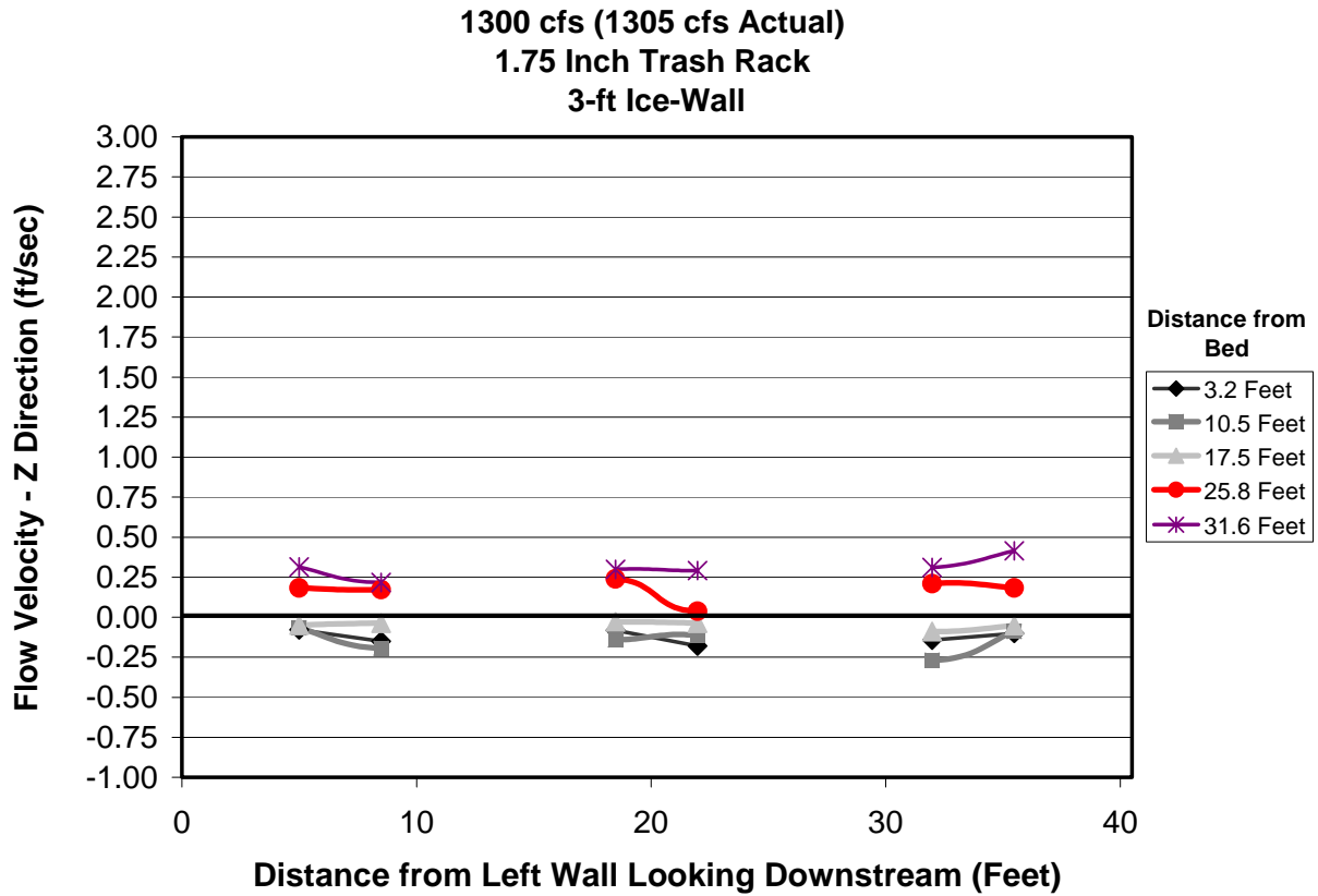
Figure C.17. The z-component of the velocity measured at 30 locations inside the bay areas, 2.9 ft away from a trash rack with 1.75-inch openings at its current location, under the 1300 cfs flow condition. The actual measured flow was 1305 cfs. The ice-wall was submerged 3-ft under normal water level conditions.
