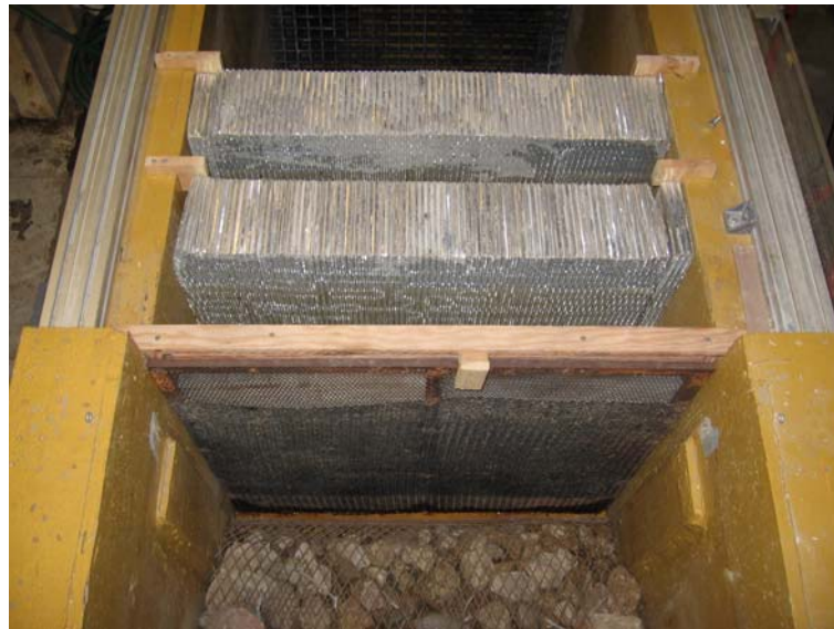
Figure 12. To dissipate the large eddies formed in the head box, wire mesh and two honeycomb screens were installed downstream of the rock crib.
