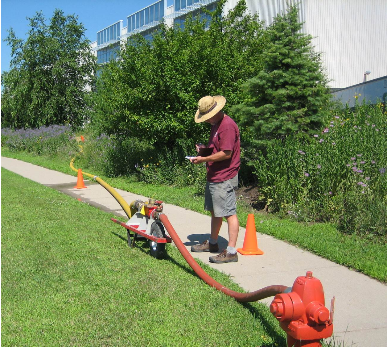
Figure 3: Adding synthetic runoff to the rain garden using a fire hydrant, fire hose, and flow meter.
