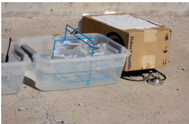
Figure 7. Photo-irradiation setup for photodegradation treatment with temperature sensor shown at the far left, “Exp” quartz flasks submerged in water bath at center, and irradiation sensor shown in lower right.
