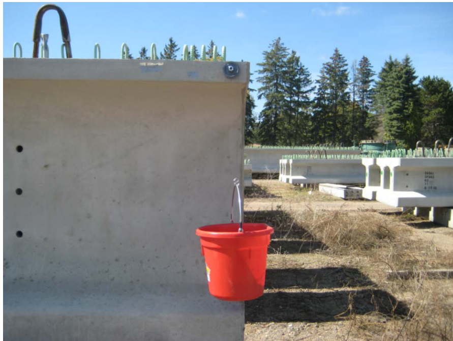
Figure 4-1. Free end of stretch-wire system with weight and pulley
