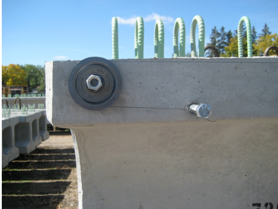
Figure 4-2. Anchored end of stretch-wire
