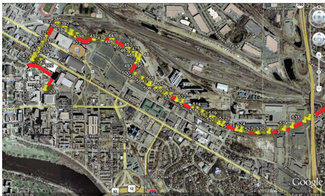
Figure 1.3: Portions of the Trip Testing Signal Outage in a Typical Urban Environment (Minneapolis/St. Paul, MN); Placemarks Show the Outbound Leg of the Test Route, with Thick Solid Lines Indicating Data Loss
