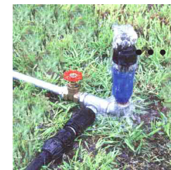
18.2 Water Pump Hydraulic ram pump
