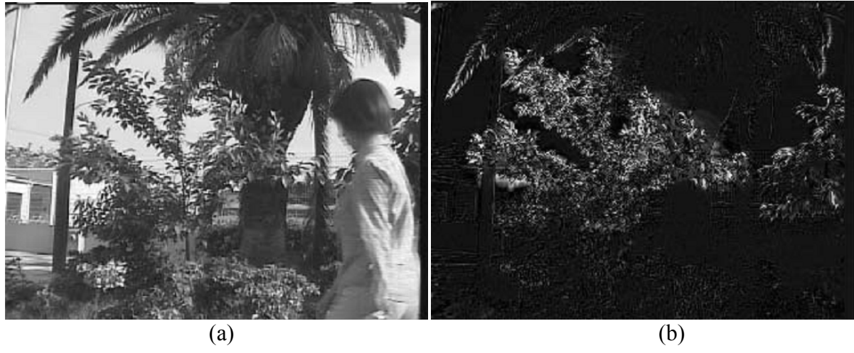
Figure 2.2. (a) A scene with waving trees; (b) Number of Gaussian distributions used to model the background pixel-wise (whiter means more and darker less).
