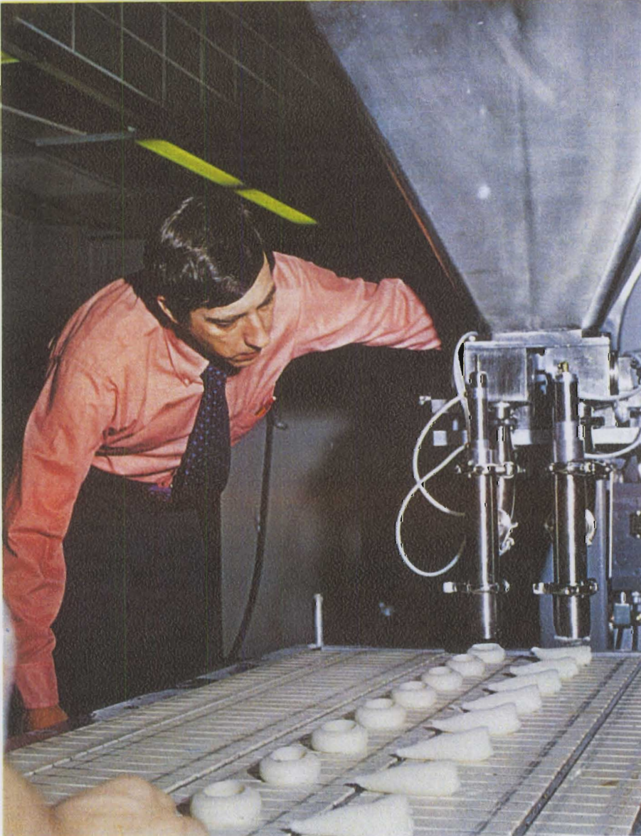
UW food scientists use a commercial extruder to dispense minced fish into various shapes. Such formed portions can be produced at rates up to 140 pieces per minute.
