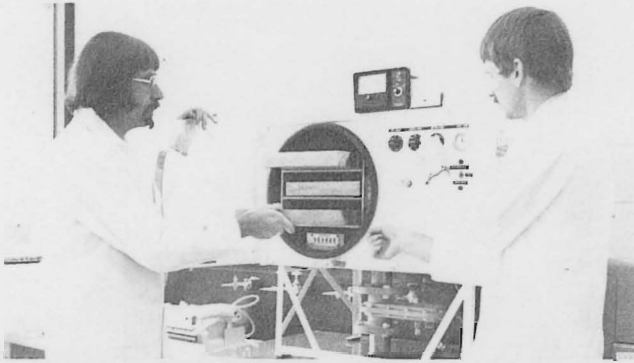
A freeze drier is readied by food scientist Ted Labuza (left) and research fellow Henry Warmbier to adjust moisture levels in food. Labuza aided in the development of several intermediate moisture foods being tested in the nation's space program.
