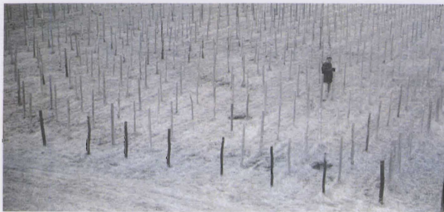
Plot for testing service life of treated and untreated posts.
