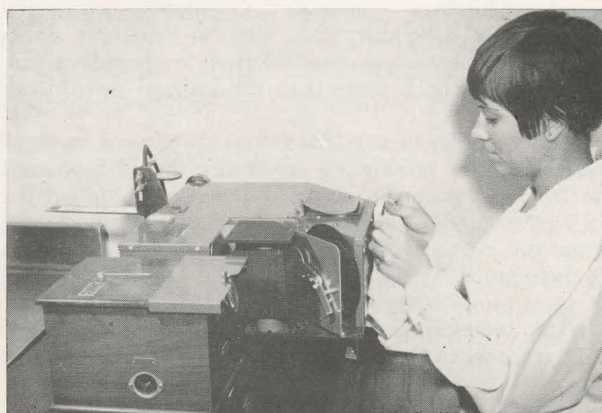
This reflectometer measured discoloration of the slips.
