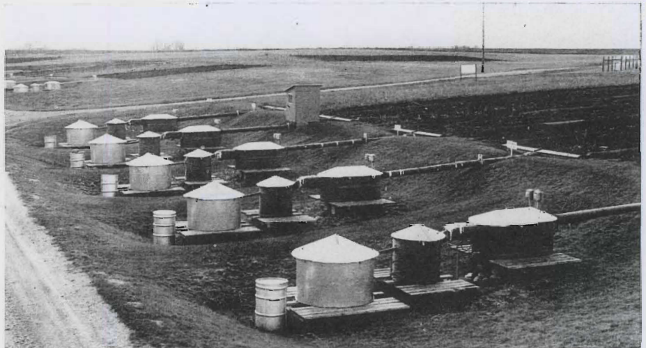
Water Conservation Research Association Farm near Morris, Minnesota. The tanks are insulated and equipped with heat cables and tank heaters to allow snowmelt runoff measurements.
