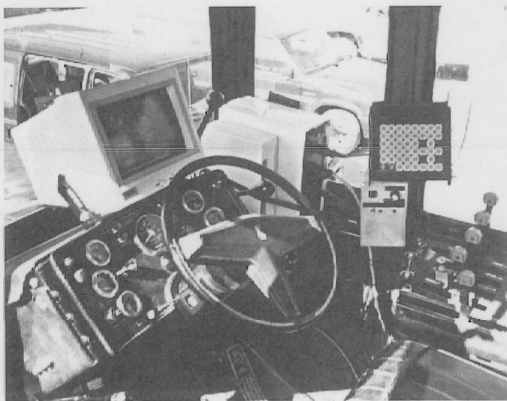
Technology in the form of Differential Global Positioning Systems guides appropriately equipped tractors with the precision that makes variable rate applications of fertilizer possible.
