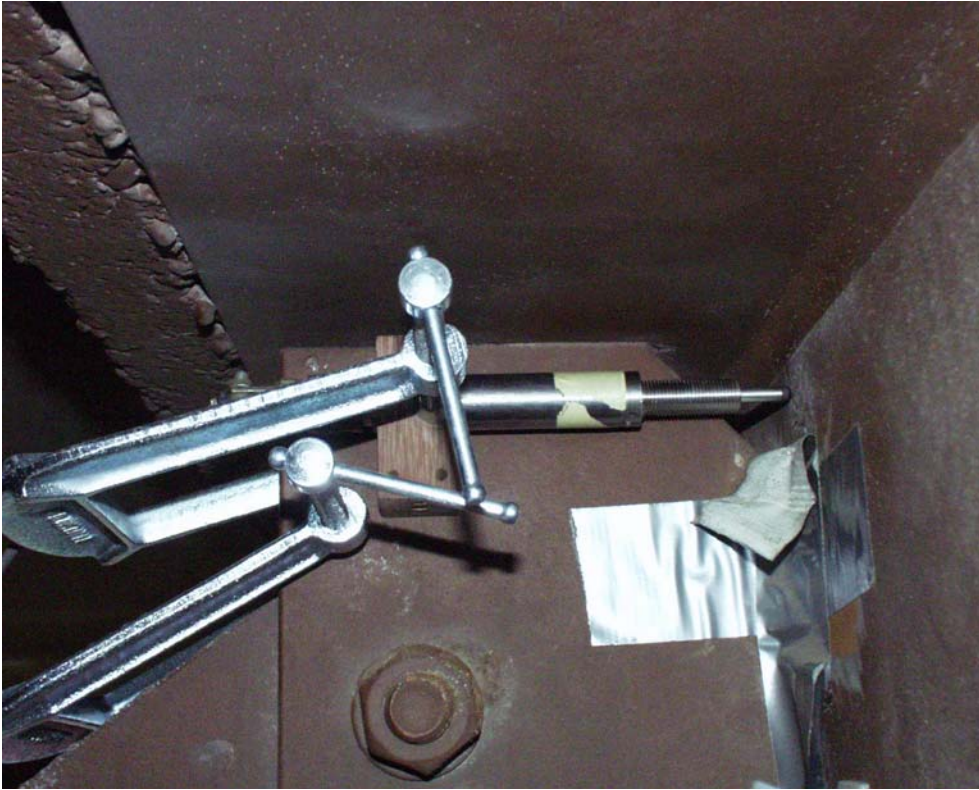
Figure 3.5 LVDT Placement for Measuring Relative Horizontal Deflection
