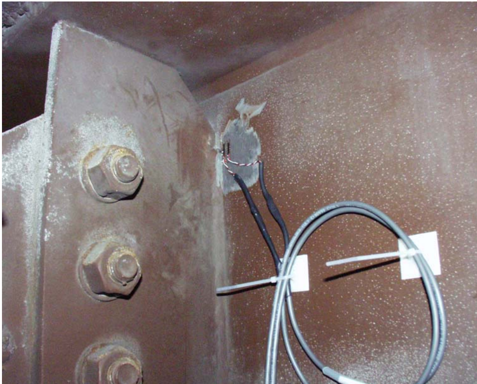
Figure 3.4 Field Placement of Strain Gages
