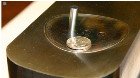
Figure 5.1: Photograph of the roughness element (which is actually a micrometer head) in the wind tunnel wall (Wheaton (2009)).
