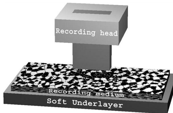
Figure 2. 2 Illustration of a perpendicular recording system using a single pole head and a perpendicular medium with soft underlayer. [2.2]
