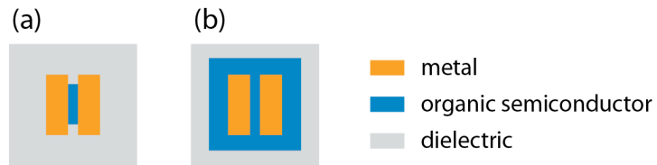
Figure A-5 OFETs for displacement current measurement. (a) The organic semiconductor film is properly patterned. (b) The organic semiconductor film is not properly patterned.
