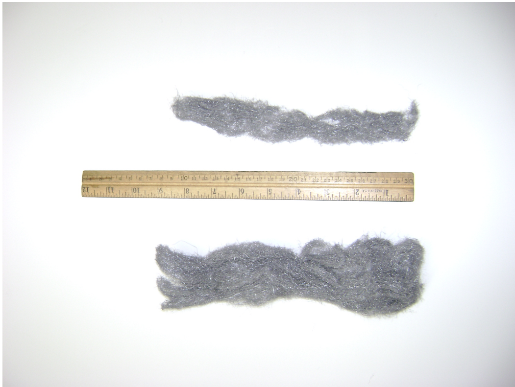
Figure 4.6: A photograph of the two meshes used in the low-power, dual-pump solid-piston experiments.
