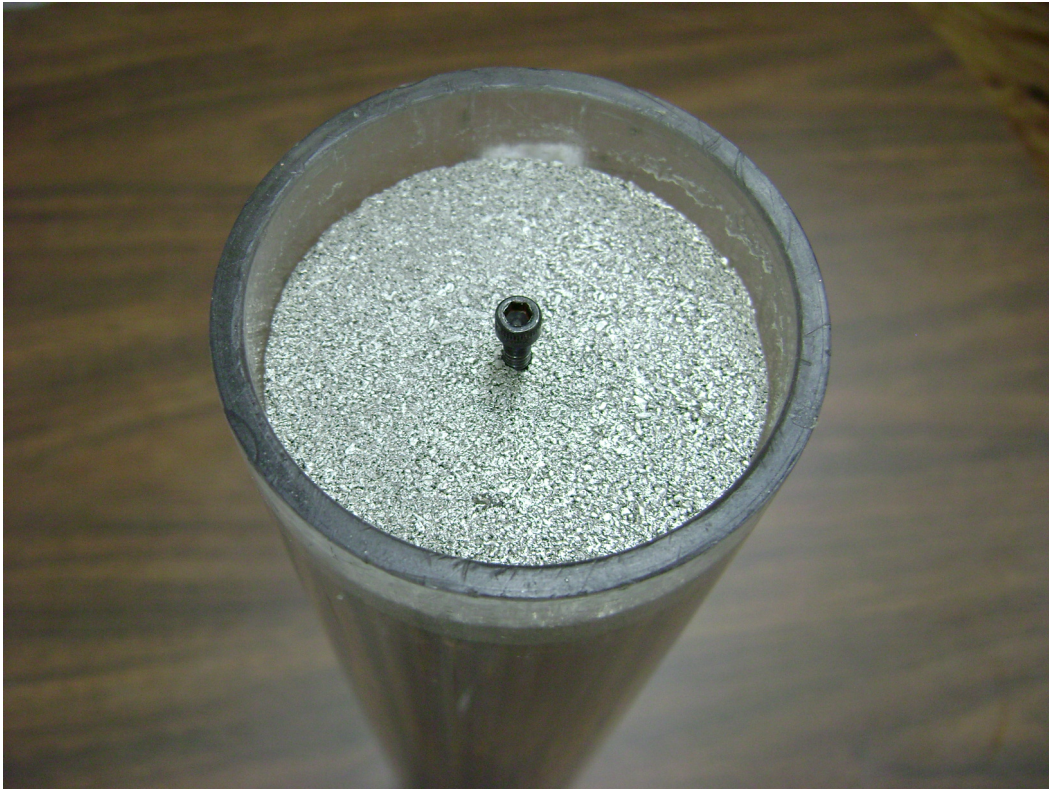
Figure 4.13: A photograph of the porous disk on top of the minitube structure. This disk prevented water from impacting the thermocouple measurements. The screw functioned as a handle so the disk could be removed. Before operation, the edges were sealed by hot glue.
