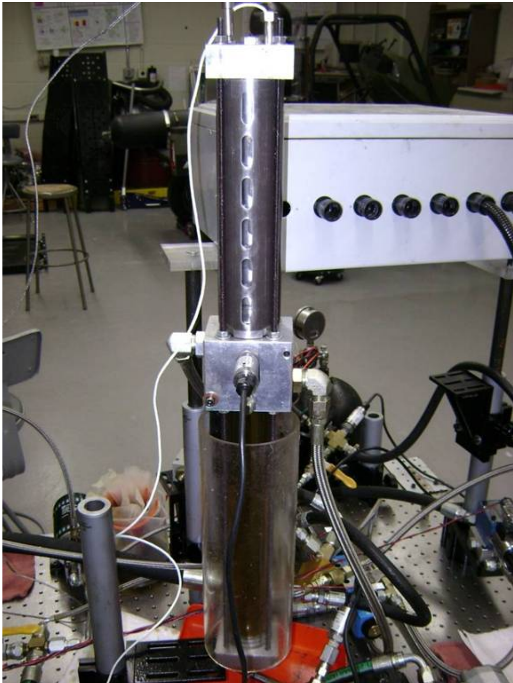
Figure 4.5: A photograph of the tandem piston-in-cylinder compressor for the low-power porous mesh experimental program.
