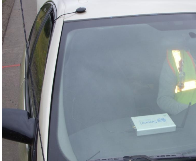
Figure 4.1 The Placement of the OBU in Test Drive Vehicle
