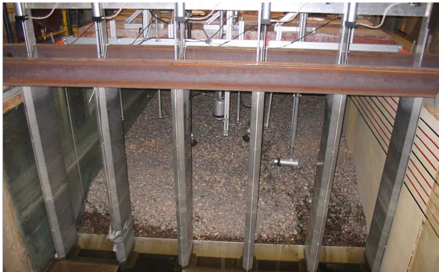
Figure 2.1: Weighing pans located at the downstream end of the experimental Main Channel.
