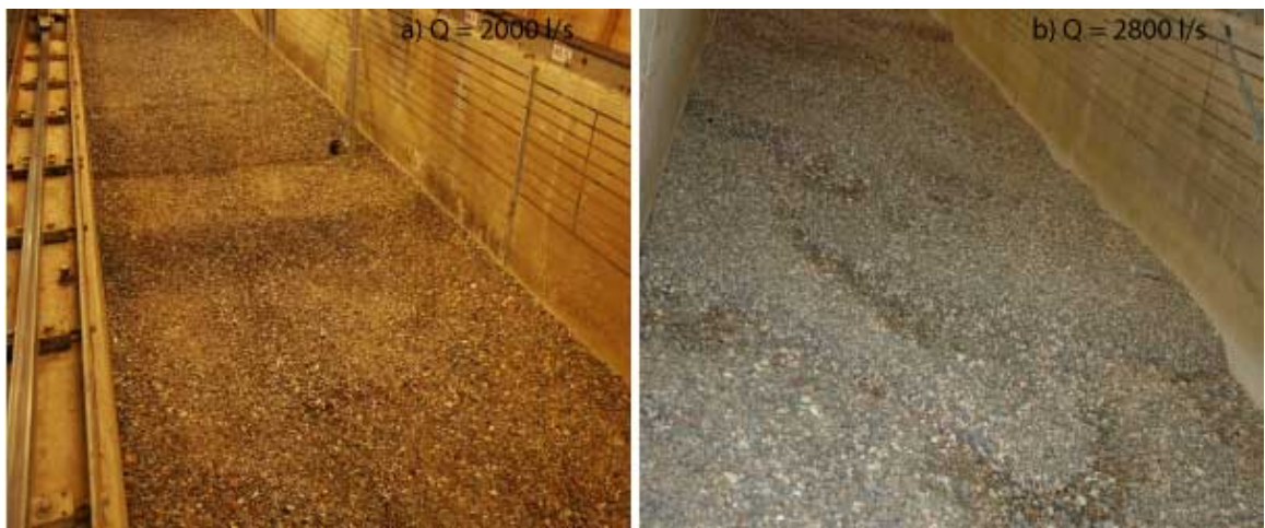
Figure 4.2: Photograph of bed surface at the end of the flow for the discharges of 2000 l/s (left), and 2800 l/s (right). The direction of flow in both cases is from the top to the bottom of the figures.
