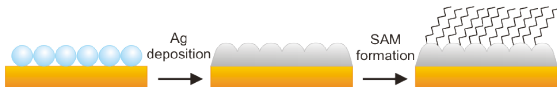
Figure 4.1 A diagram demonstrating the fabrication process of the partition-layer modified AgFON. First, silica spheres are packed on clean copper disks, then 200 nm of Ag is deposited onto the nanosphere mask, and then the monolayer is formed during exposure of the substrate to an ethanolic alkanethiol solution.
