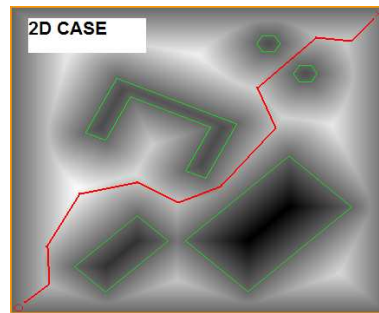
Figure 3.4: Motion planning using potential fields
