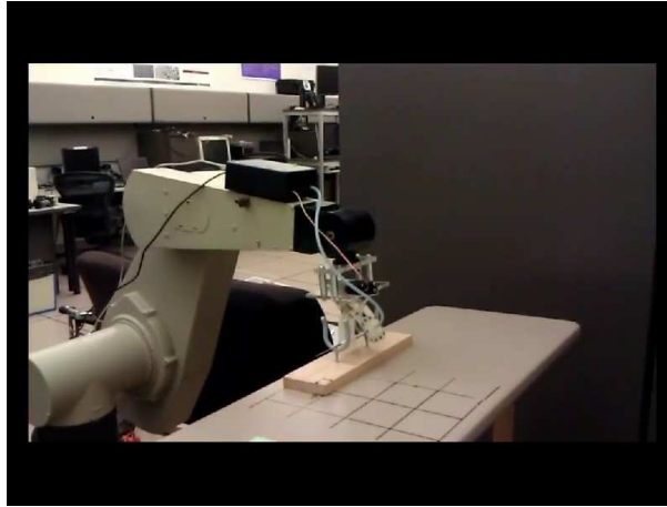
Figure 8.3: Loading instrument from tray
