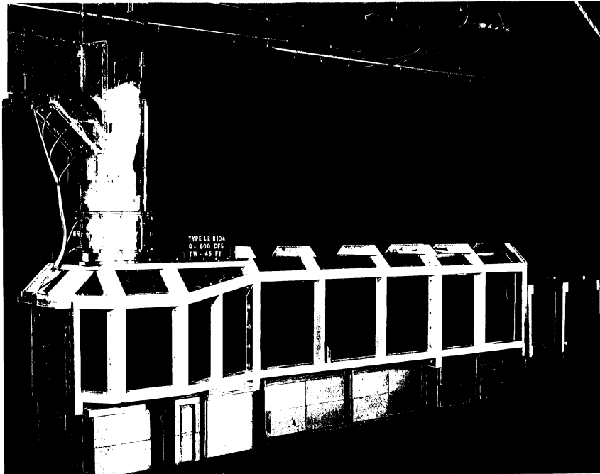
Photo 55. Type L2 R104 dropshaft, Q = 600 cfs, T.W. = 45 ft. The final design.
